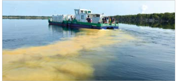
LMBV remediation ship "Klara" being used for the improvement of the water quality of post-mining lakes
